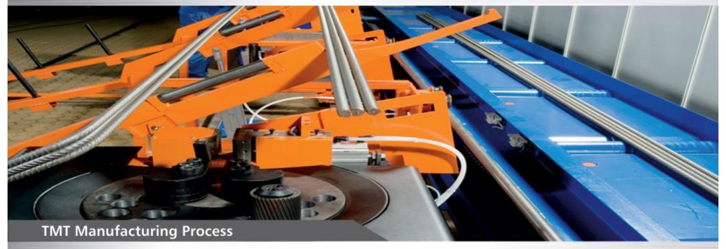
This process is widely accepted as the best process for production of high quality rebars since the technology uses low cost raw materials against costly alloy elements like Vanadium and Niobium, but results in the same high mechanical properties (DIN 488 IVS, BS 4449:97 etc.) ensuring excellent weldability, ductility and bendability a notable saving in alloy cost per ton.
